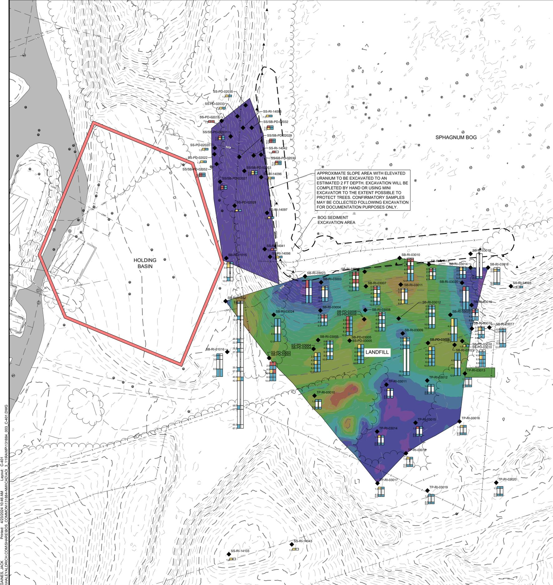
APPROXIMATE SLOPE AREA WITH ELEVATED URANIUM TO BE EXCAVATED TO AN ESTIMATED 2 FT DEPTH. EXCAVATION WILL BE COMPLETED BY HAND OR USING MINI EXCAVATOR TO THE EXTENT POSSIBLE TO PROTECT TREES. CONFIRMATORY SAMPLES MAY BE COLLECTED FOLLOWING EXCAVATION FOR DOCUMENTATION PURPOSES ONLY.
