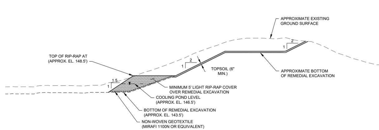
**2** TYPICAL CROSS SECTION AT SECTION 2
