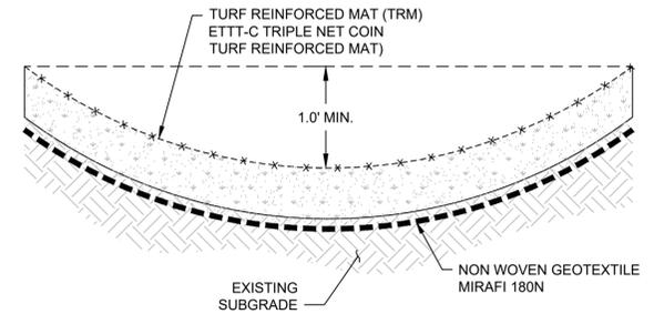
**7 TURF - REINFORCED MAT (TRM) SWALE DETAIL**
