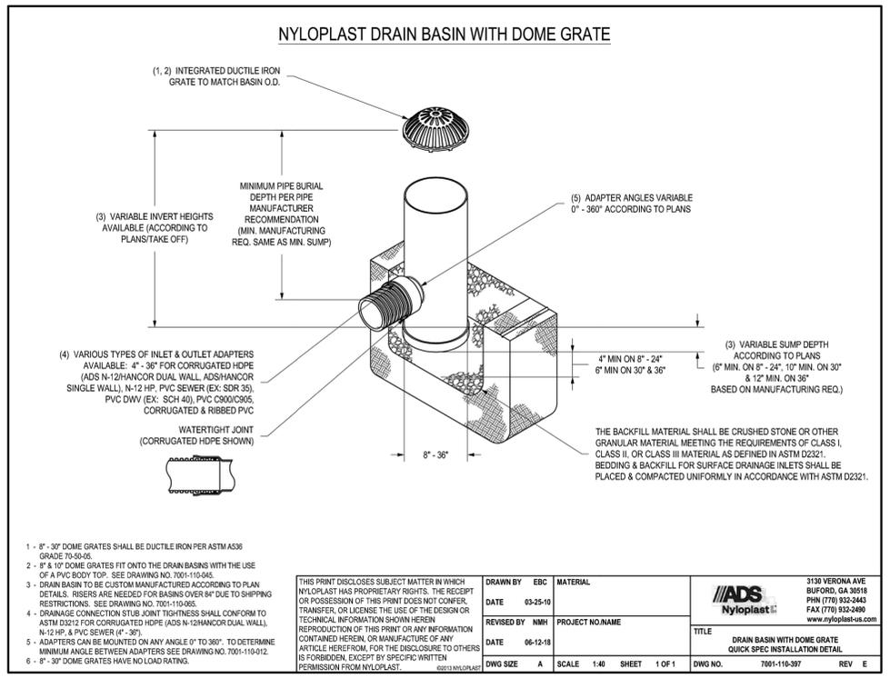
**6 NYOPLAST DRAIN BASIN WITH DOME GRATE DETAIL**
