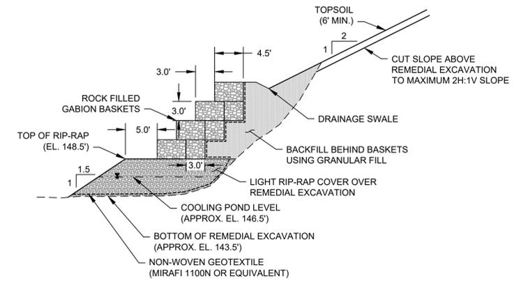
**3** TYPICAL CROSS SECTION AT SECTION 3
