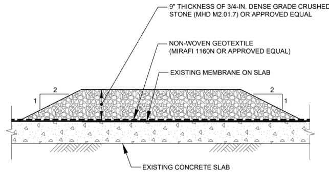
**2 PROPOSED TRUCK ROADWAY OVER EXISTING BUILDING SLAB**
