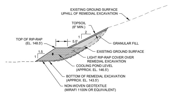
**5** TYPICAL CROSS SECTION WITH FILL TO FLATTEN SLOPE
