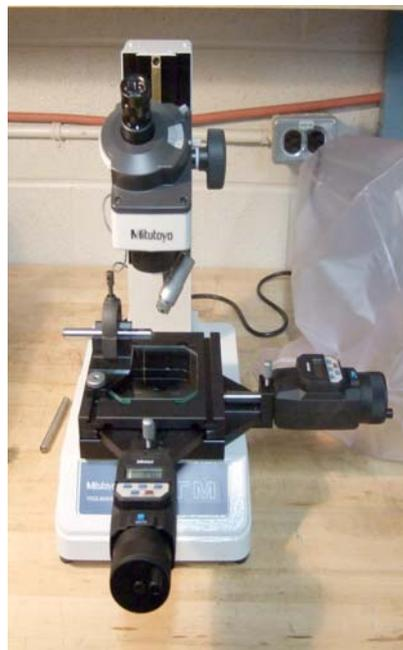
FIG. 2 Toolmaker's Microscope
