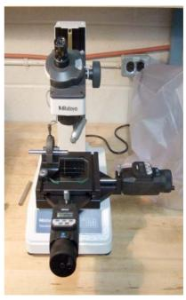
FIG. 2 Toolmaker's Microscope
