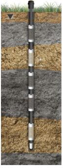
Typical 3-Channel CMT Installation in Overburden with Bentonite and Sand Cartridges
