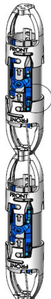
FIGURE 1 , example with 2 of the VOA-size Snap Sampler Modules. Up to 6 modules can be assembled in any combination of sizes.
